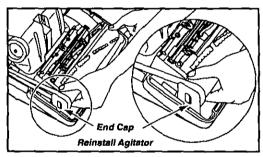
After checking the end caps, reinstall the agitator brush assembly back into the housing grooves After installing the agitator brush assembly, turn it by hand making sure that the belt is not twisted or pinched and all rotating parts turn freely. Replace the lower plate as described in the REMOVING/INSTALLING THE LOWER PLATE section
