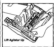
Remove the agitator brush assembly, (carefully lift it out), and remove the worn or broken belt from the agitator pulley and motor shaft
