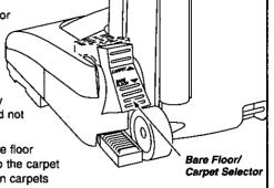
Take care when selecting either position to make sure the selector is pushed fully and quickly as possible to the desired position. Failure to do so can cause the belt to rub on the selector shaft and may result in the belt becoming hot and creating a burning rubber smell
